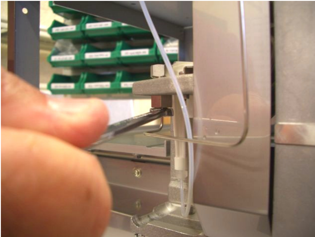
Figure 4: Loosening the Bottom Fittings on the injection port
